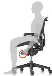
Engage the tilt limiter when you want to sit in an upright or partially reclined position.
